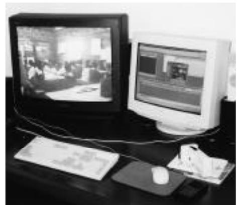
*Pictured is a non-linear desktop video editing system. The screen on the right displays the computer programme that is being used to edit the video. The screen on the left allows the viewer to see the output during the editing process.*
