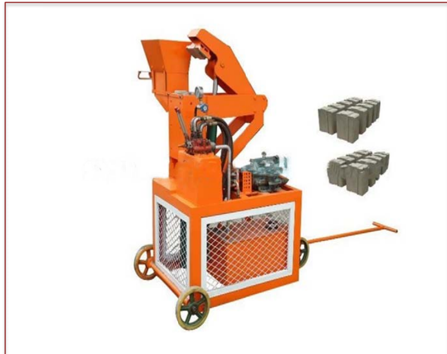
Figure 3: Single mode motorised soil compacting machine.
