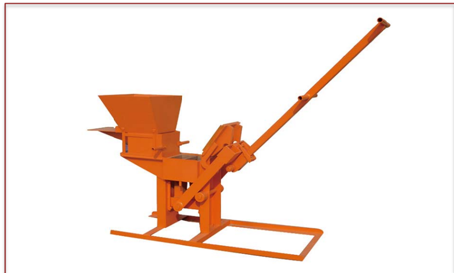
Figure 2: Manually operated interlocking block machine.
