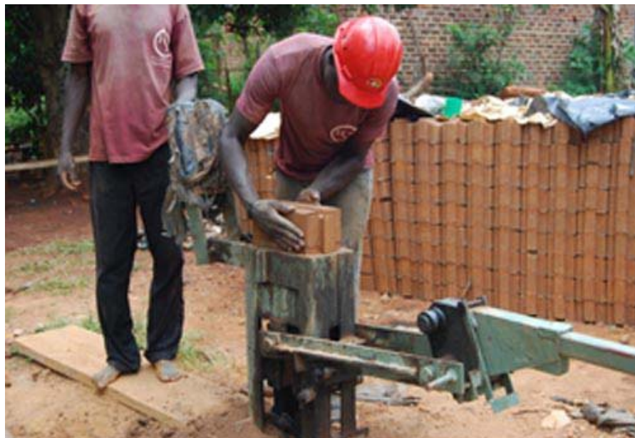
Figure 11: Removing the block from the machine.
