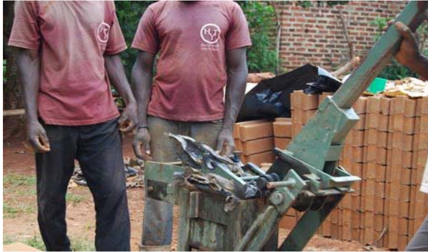
Figure 9: Block compacting machine.
