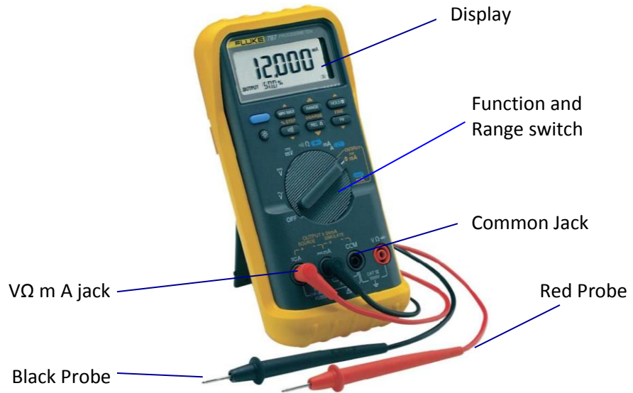
Figure 29: Parts of a multimeter
