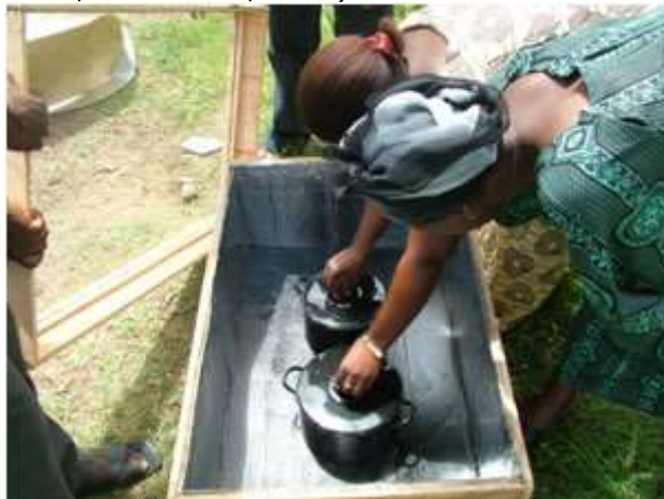
Figure 2: Box Solar Cooker with Glass Lid, Ago-Are, Nigeria (with Rukayat Adewumi, front, and Grace, back)
