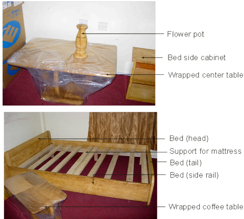
Fig. 4 Photograph of center table, flower pot, bedside cabinet coffee table, and bed manufactured from oil palm wood
